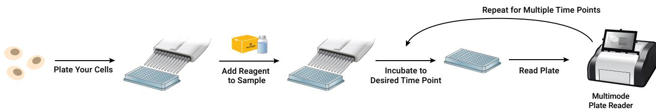
Plate your cells and add the reagent directly to the cells only once. The assay can be performed without further washing or processing steps. Read the plate at each time point, as many times as you need!
