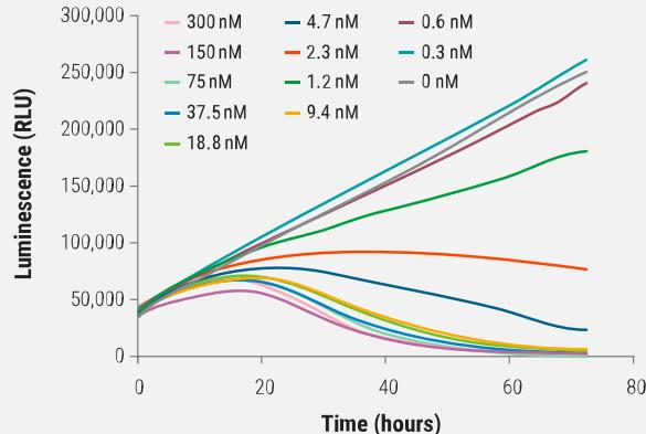
A549 cells (500 cells/well) were plated in medium containing the RealTime-Glo™ Reagent in 384-well plates. Cells were treated with bortezomib at the indicated concentrations and monitored every hour for 72 hours.
