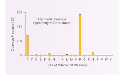
Human K562 extract was digested with ProAlanase at pH 1.5 for 2 hours at 37°C using a 1:100 enzyme:substrate ratio. Peptides were analyzed by LC-MS/MS on a Q-Exactive Plus. Data were searched using Byonic $^{\text{TM}}$  software with no enzyme specified.
