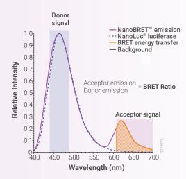
Measuring PPIs in living cells with NanoBRET™ Technology requires the expression of the two interacting proteins of interest (A, B) as fusion proteins with either NanoLuc® luciferase or the HaloTag® protein, respectively. If the interaction partners are in close proximity (< 10 nm), the NanoBRET™ 618 fluorophore will be excited by the NanoLuc® luciferase via BRET.
