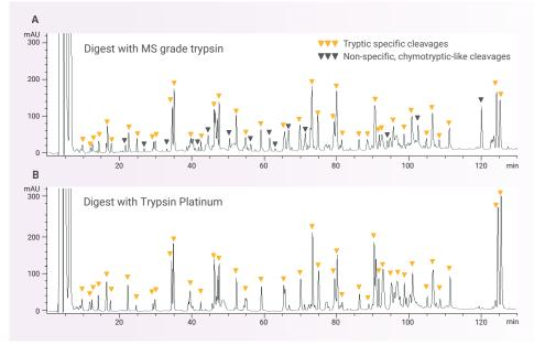
Trypsin Platinum (Panel B) is free of non-specific cleavage activity compared to MS grade trypsin (**Panel A**). Panitumumab (Vectibix®) antibody used as a model protein substrate was digested with MS grade trypsin and Trypsin Platinum. The digestion reactions used a 1:10 trypsin:protein ratio. The digests were analyzed with RP-HPLC-UV
