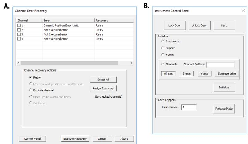
**Figure 22. Error caused by a physical obstruction detected by the intrusion sensor. Panel A.** When the intrusion sensor on the Maxprep® Liquid Handler detects a physical obstruction that would impede gantry movement prior to gantry motion, the error above is displayed. **Panel B.** Follow the instructions in the text above to reinitialize the instrument and continue processing.
