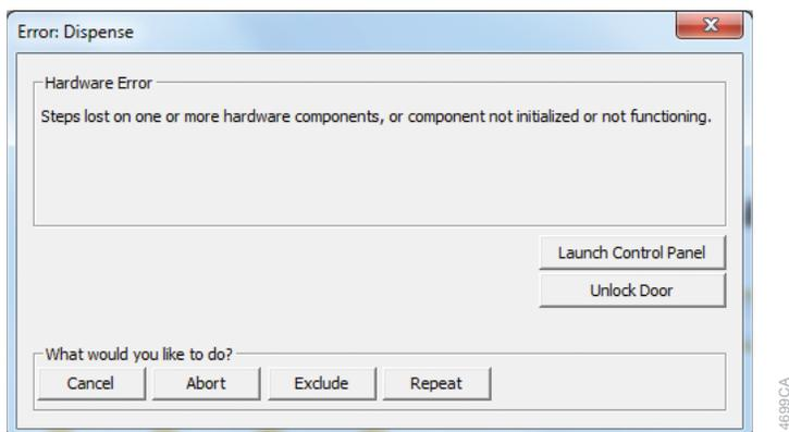
**Figure 25. Hardware Crash.** In the event that there is a physical crash of hardware components that results in an error message, press the **Abort** button on the error screen to end the method run.
