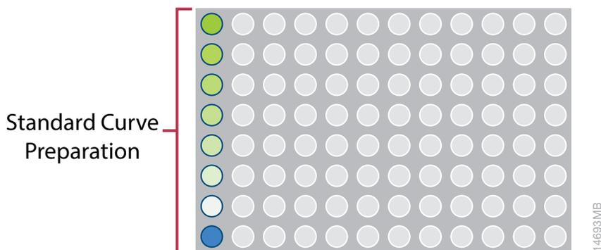
**Figure 19. Standard Curve Labware.** The standard curve labware is used to prepare standard curve serial dilutions. Place a PCR plate or strip tube in the first column of an amplification plate base at Site 1 of the Tip and Plate Carrier (shown in Figure 18).
