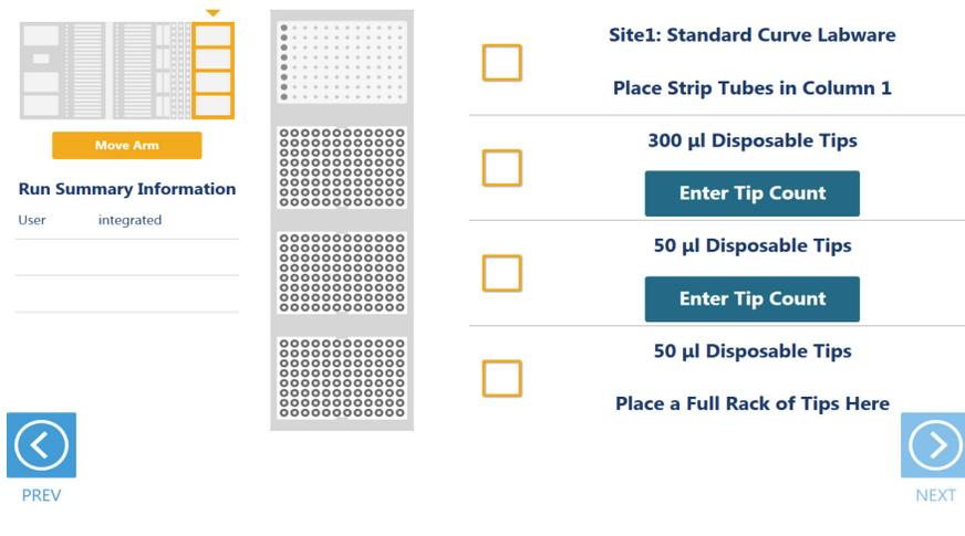
**Figure 18. Tip and Plate Carrier screen.** Place the specified labware at each site. Site 1 contains either an amplification plate or strip tubes in the first column of an amplification plate base. Sites containing a tip rack indicate the type of tips that should be placed there and whether a partial or full rack of tips needs to be placed. For partial tip racks, press the **Enter Tip Count** button to specify the first available tip in the partial tip rack
