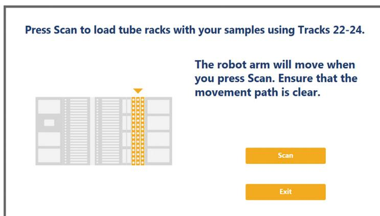
**Figure 8. Scanning tube racks.** Tube racks at Tracks 22–24 must be scanned when tubes are selected as an input labware type. Scanning tube racks will determine the type of tube rack being used, the types of tubes defined for the rack type and the sample identifiers for each tube.
