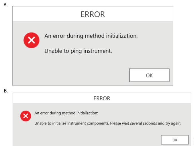
**Figure 27. Instrument Connection Errors.** Connection errors will be displayed during a run if the instrument has not completed its full internal initialization before a method run is started. The errors shown in **Panels A** and **B** may be displayed. Confirm that the instrument is powered on and has fully initialized, then press the **OK** button, wait several seconds and attempt to restart the method.
