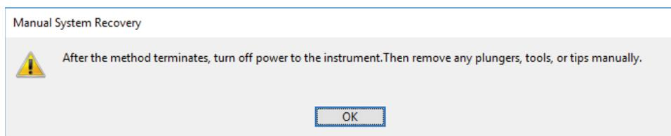
**Figure 26. Aborted Method.** A message will be displayed after aborting a run indicating that the instrument should be powered off. After turning the instrument off, open the door and manually resolve the crash state as instructed in the *Maxprep® Liquid Handler Technical Manual #TM509*. After any instrument crash, contact Promega Technical Services to determine whether the instrument may require a service visit.
