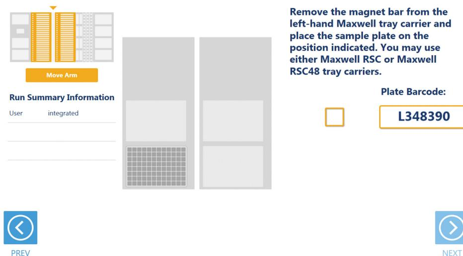
**Figure 15. Sample Plate Position.** When using a plate as input labware, the plate is placed on the front plate position of the left Maxwell® Deck Tray Carrier as indicated. Any type of Maxwell® Deck Tray Carrier can be used. Remove any Maxwell® deck tray and the elution magnet from the Maxwell® Deck Tray Carrier before placing the sample plate.
