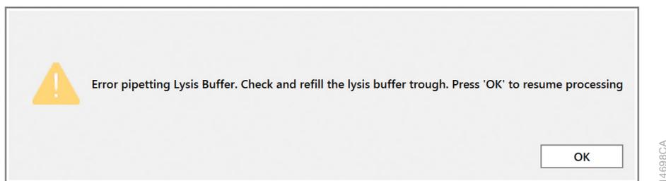
**Figure 24. Insufficient reagent on the system to complete a method.** In the event that insufficient reagent is detected in a trough or tube position, a warning will be displayed; the instrument will pause and unlock the door. Open the door, replenish the indicated reagent, close the door and press **OK** to resume processing.
