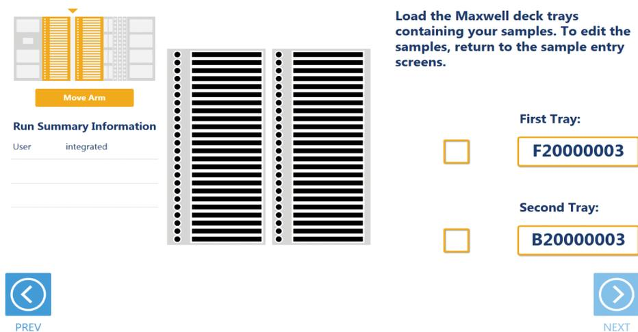
**Figure 14. Maxwell® Deck Tray Carriers.** These carriers are used to hold 16-position Maxwell® deck trays or 24-position Maxwell® deck trays (Front and Back). Place Maxwell® deck trays with elution tubes at the indicated positions on the deck tray carriers as instructed.
