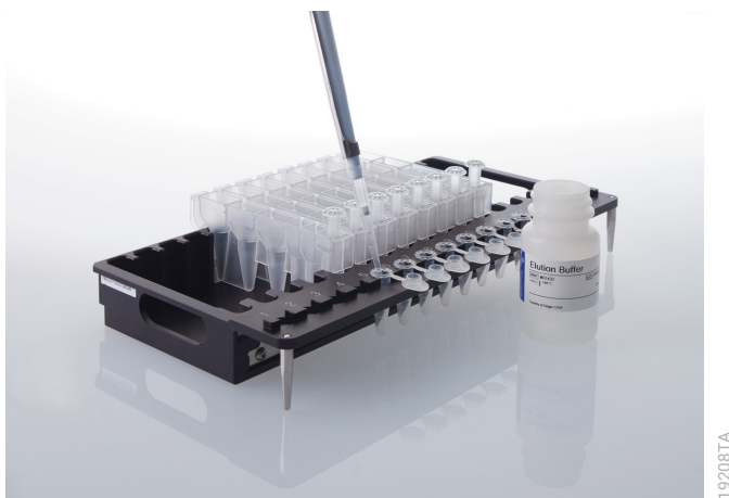
Figure 3. Setup and configuration of the deck tray(s). Elution Buffer (RCFD) is added to the elution tubes as indicated. Plungers are in position #6 of the cartridge. Deck tray shown is from the Maxwell® RSC Instrument (Cat.# AS4500).
