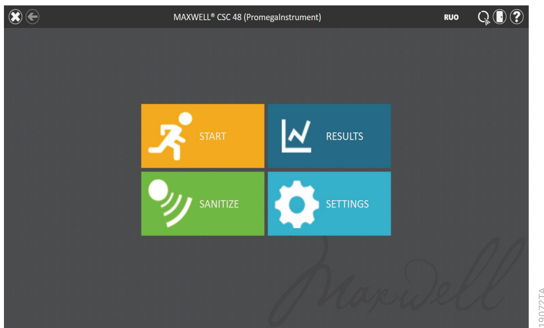
Figure 37. Maxwell® CSC 48 'Home' screen. When the Quantus™ Fluorometer is correctly connected to the Maxwell® CSC 48 instrument, the “Q” logo is displayed in the upper right corner of the title bar.
