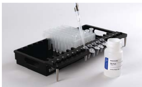
Figure 2. Setup and configuration of the Maxwell ® CSC Deck Tray. Nuclease-Free Water is added to the Elution Tubes as indicated.
