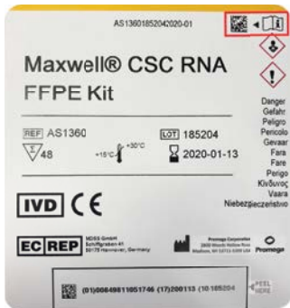
Figure 3. Kit label indicating the method bar code to scan. Shown in the red box is the method bar code to scan on the kit label for starting a purification run.
