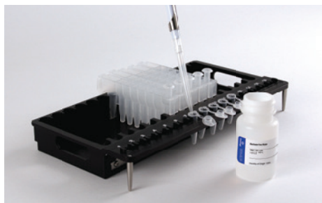
Figure 2. Setup and configuration of the deck tray(s). Elution Buffer is added to the elution tubes as shown. The plunger is in well #8 of the cartridge.
