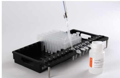
Figure 2. Setup and configuration in the deck tray(s). Elution Buffer is added to the Elution Tubes as shown. Plungers are in well #8 of the cartridge.
