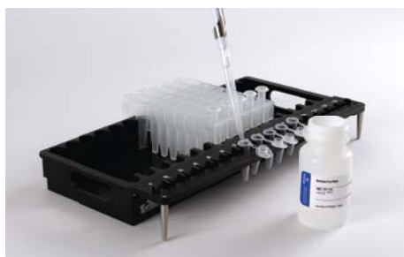
Figure 2. Setup and configuration of the deck tray. Elution Buffer is added to the elution tubes as shown. Plungers are in well #8 of the cartridge.
