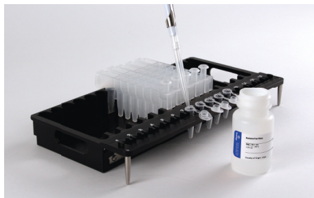
Figure 2. Setup and configuration of the deck tray(s). Elution Buffer is added to the elution tubes as shown. Plungers are in well #8 of the cartridge.
