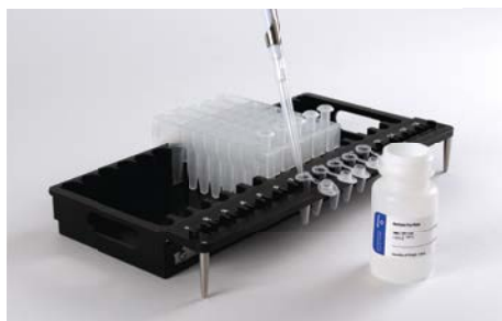
Figure 2. Setup and configuration of the deck tray(s). Elution Buffer is added to the elution tubes as shown.
