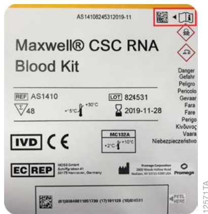
Figure 3. Kit label indicating the method bar code to scan. The red box and arrow at the top of the label highlight the method bar code on the kit label. Scan this bar code to start a purification run.
