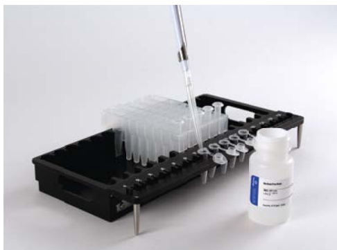
Figure 2. Setup and configuration of the Maxwell® CSC Deck Tray. Nuclease-Free Water is added to the Elution Tubes as indicated.
