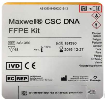
Figure 3. Kit label indicating the method bar code to scan. Shown in the red box is the method bar code to scan on the kit label for starting a purification run.
