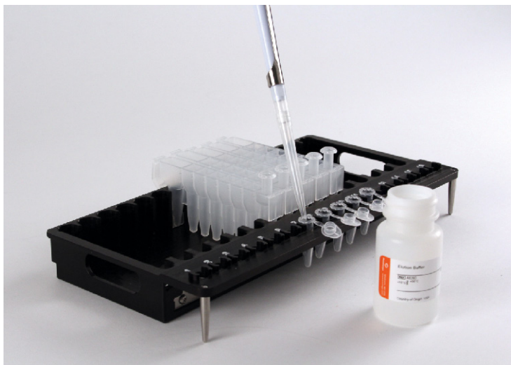
Figure 2. Setup and configuration of the deck tray. Elution Buffer is added to the Elution Tubes as indicated.
