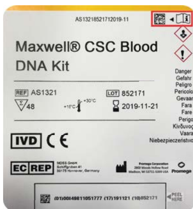
Figure 3. Kit label indicating the method bar code to scan. Shown in the red box is the method bar code to scan on the kit label for starting a purification run.
