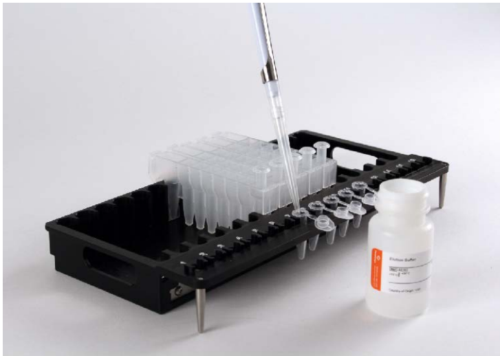
Figure 2. Setup and configuration of the Maxwell® CSC Deck Tray. Elution Buffer is added to the Elution Tubes as indicated.
