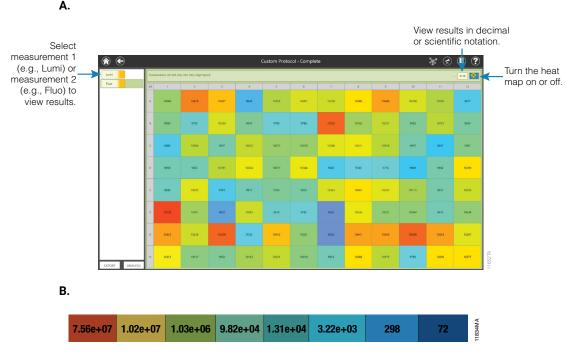
Figure 55. Results plate map with heat map display (Panel A) and example of heat map colors applied to the results in the plate map (Panel B).
