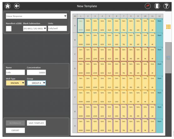
**Figure 71. Multiple experimental data sets.** When creating an analysis template with multiple experimental data sets, select all the wells that are part of each data set (containing Known, Unknown and Blank wells that should be analyzed together) and assign a group from the Group drop-down menu. A unique color will be applied to each group.
