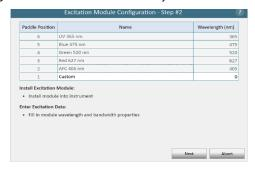
Figure 93. Setting name, wavelength and bandwidth.
