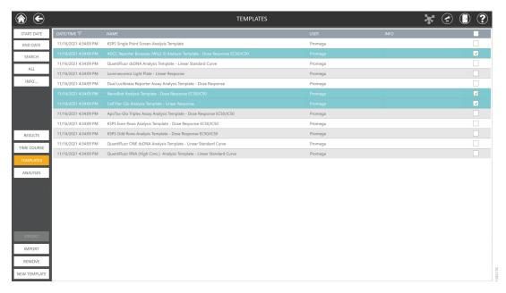
Figure 61. Functions of the 'Results, Time Course, Templates and Analyses' screen. From the 'Results, Templates and Analyses' screen, you can **Export** or **Remove** one or more list items, **Import** a result, template or analysis (.raw, .template, .analysis) file or create a **New Template**.
