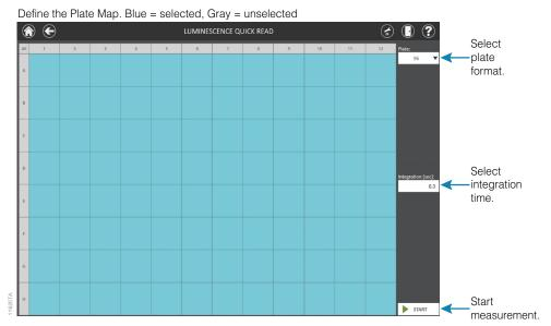
Figure 11. GloMax® Discover 'Luminescence Quick Read' screen.
