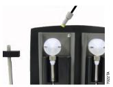
Figure 115. Attaching the fitting to the inside port.
