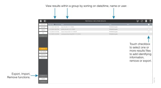
Figure 63. The 'Results, Templates and Analyses' screen.
