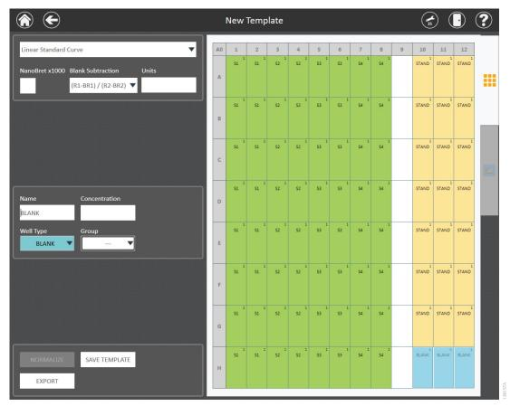
**Figure 68. Well naming.** Well names assigned to individual wells. S1-S4 names have been assigned to Unknown wells containing replicates of individual samples. STAND name has been applied to the replicates in the standard curve, and BLANK has been assigned to the Blank wells.
