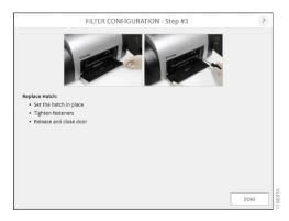
Figure 91. Replacing the hatch door.
