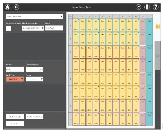
**Figure 74. Control well assignment.** A Control well type must be assigned in order to perform data normalization to % Control or Fold Change. The **Normalize** button becomes active once a Control has been assigned to the plate.
