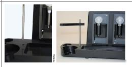
Figure 116. Inserting the vertical support rod and inlet tube holder.
