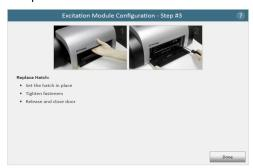
Figure 94. Replacing the hatch door.
