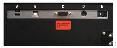
**Figure 5. The back of the GloMax® Discover Instrument. A**. Two USB ports to attach an external USB flash drive, USB hub or Bar Code Reader. **B**. USB port to connect to Tablet PC. **C**. Injector System connection. **D**. Power connection. **E**. On/Off switch.
