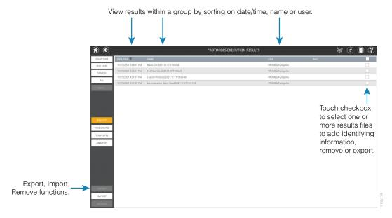
Figure 60. 'Results, Time Course, Templates and Analyses' screen functions. This screen is used to display Results that have been generated, analysis Templates and data Analyses. Export, Import and Remove buttons in the lower left corner of the screen can be used to perform their indicated functions.
