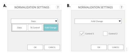
Figure 75. Data normalization. Panel A. There are two options for data normalization, % Control and Fold Change, and an option to undo normalization, Data. After selecting the normalization mode, normalization will automatically assign the control that is present on the plate. Panel B. If there are two controls on the plate, the user must specify which control to use for normalization.
