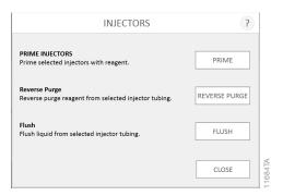
Figure 120. Injector functions (prime, reverse purge and flush).
