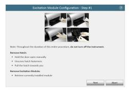
Figure 92. Custom Fluorescence Excitation Module configuration procedure.
