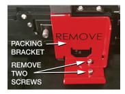
5. After removing the red Packing Bracket, remove the blue Packing Bracket Mount, and ensure the instrument is free of any packaging material parts.
