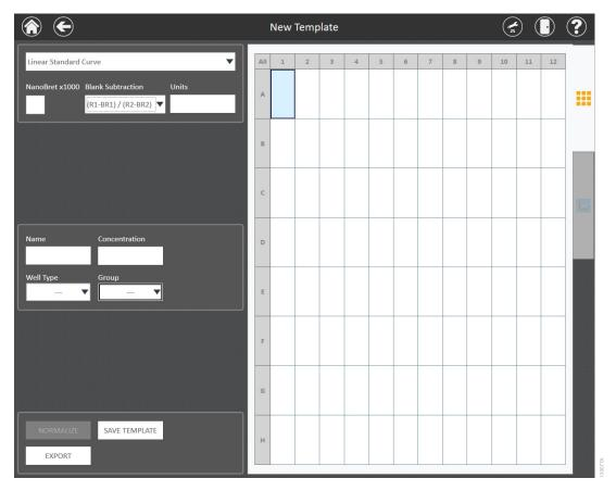
Figure 66. New Template creation. From this screen, the user will define the curve fit type, units, well types, concentrations/dilution factors and names in the analysis template.
