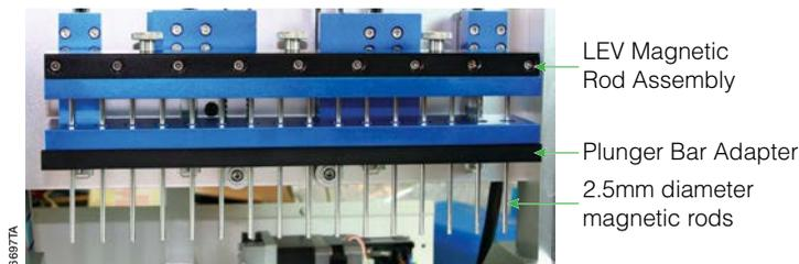
**Figure 2. Maxwell® 16 Instrument hardware set to LEV configuration.** Refer to the *Maxwell® 16 Instrument Operating Manual* to reconfigure your instrument to the LEV hardware configuration.
