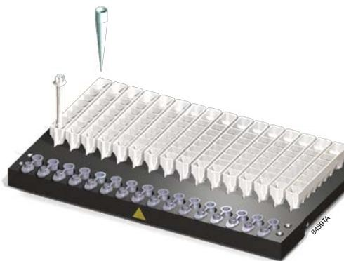
2. Place a plunger into Well #8 of each cartridge with the tabs sticking up. (Well #8 is the well closest to the elution tube).
