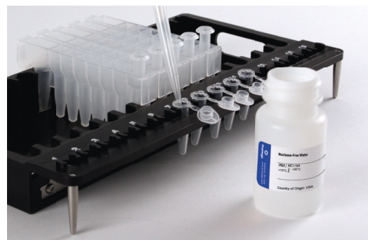
Setup and configuration of deck trays. Nuclease-Free Water is added to the elution tubes as shown. Plungers are in well #8 of the cartridge.
