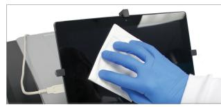
4. To clean the Tablet PC, turn OFF the power. Use a Kimwipes® tissue dampened with 70% ethanol to gently and cautiously clean the touch screen.
