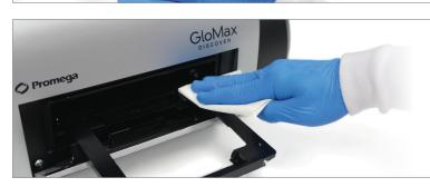
**3.** Use a cloth dampened with deionized water to periodically wipe clean the exterior of the instrument.
