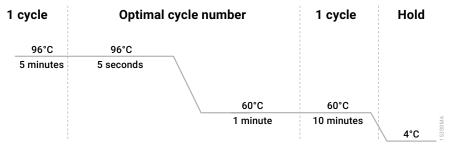
Figure 1. The thermal cycling protocol for the ProFlex® PCR System, GeneAmp® PCR System 9700 and Veriti® 96-Well Thermal Cycler.
