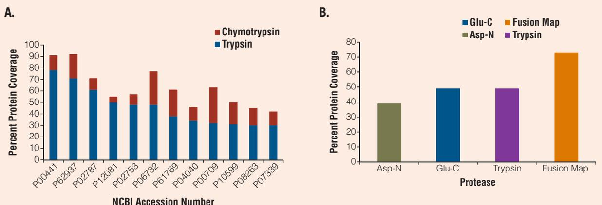
**Figure 7.7.** Increased protein coverage using (**Panel A**) both trypsin and chymotrypsin; (**Panel B**) multiple proteases in separate digestion reactions. Note that the fusion map is the combination of the results obtained by digestion with each protease alone.
