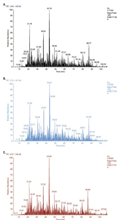
**Figure 7.17.** Lot-to-lot reproducibility. Base peak chromatograms of three different human protein extract batches analyzed by LC/MS. Each run used 1 µg of human pre-digested protein extract injected into the instrument (Waters NanoAquity HPLC system interfaced to a ThermoFisher Q Exacte). Peptides were resolved with 2h gradient.
