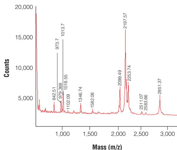
**Figure 7.2.** Spectrogram of bovine carbonic anhydrase II digested by Trypsin Gold, Mass Spectrometry Grade. A 500ng sample of carbonic anhydrase II was separated by gel electrophoresis and digested with 500ng of Trypsin Gold, Mass Spectrometry Grade, overnight at 37°C.\*
