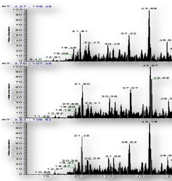
Waters NanoAquity HPLC system interfaced to a Themo Fisher Q Exactive, 2h gradient, 1 ug extract injection.
