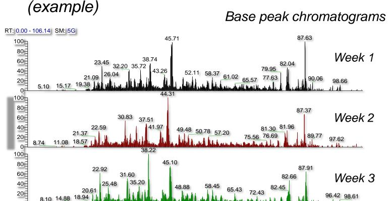
nstrument performance (Waters NanoAquity HPLC system interfaced to a ThemoFisher Q Exactive) was monitored with human pre-digested extract (1ug injection, 2h gradient).
