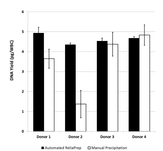
Normalized DNA yields across multiple donors for both automated and manual methods. DNA yields are normalized based on the white blood cell counts for each donor. Each bar is the mean of quadruplicate samples with error bars of one standard deviation.
