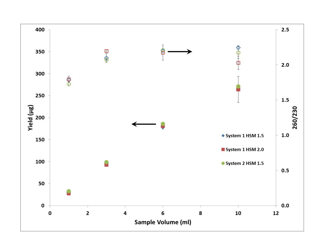
Samples from a single donor were processed on two different Tecan Freedom EVO® - HSM systems. One system is fitted with both an HSM 1.5 and an HSM 2.0. The second system is a Standard Solution configured robot equipped with an HSM 1.5.
