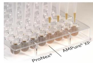
Fig 3: Comparison of retention in tips between chemistries due to viscosity of the solutions. An 8-channel pipette was used to simultaneously manually pipette both ProNex® System and AMPure XP products for one aspirate/dispense cycle of the chemistries. The volume of chemistry retained in tips is variable and noticeably higher for AMPure XP chemistry.
