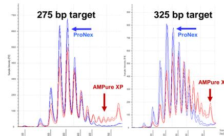
Fig 5: Comparison of ProNex® Chemistry vs. AMPure XP chemistries for size selection. A 50bp ladder was size-selected for two different library target sizes (275 and 325bp).
