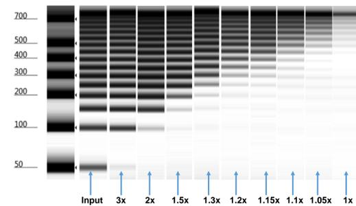
Fig. 1: Gel images demonstrating retention of varying sizes of DNA based on altering the ratio of bead volumes added to original sample volumes. Ratios and size retention shown are the result of sample cleanup of a 50bp ladder with decreasing ratios of Promega's ProNex® Size-Selective Purification System.<sup>1</sup>
