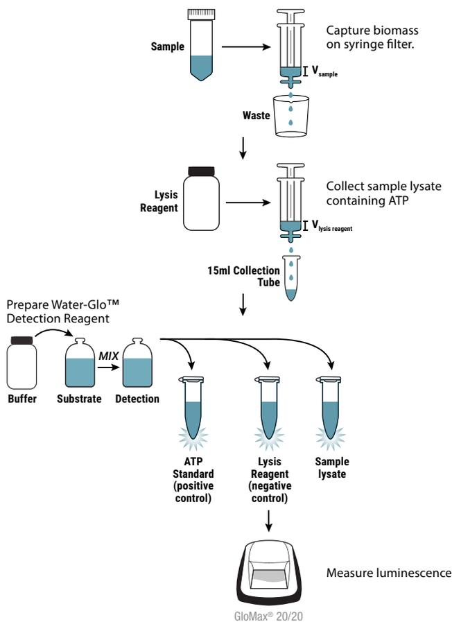
Figure 1. Procedure of Filtration Method Using the Water-Glo™ Kit.
