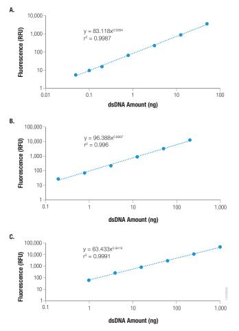
Figure 3. QuantiFluor<sup>®</sup> dsDNA Dye at three different concentrations accurately quantitates DNA over a range of 0.05–1,000ng in 384-well format. Panel A. 0.2µl dye/well; Panel B. 1µl dye/well; Panel C. 3µl dye/well.
