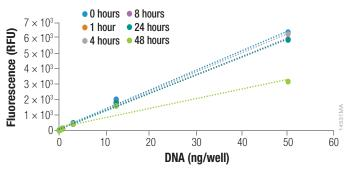
**Figure 2. QuantiFluor® dsDNA Dye working solution.** A 1:200 dilution working solution was left in a trough on the deck of a liquid handler exposed to ambient laboratory temperature and light. Dye was used at several time points to measure DNA in 384-well plate format over the range 0.05–50ng/well. A decrease in RFU signal was observed only after 24–48 hours.
