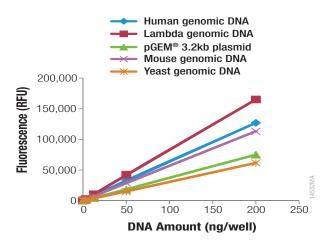
Figure 4. Five different DNA standards measured using the QuantiFluor® dsDNA System. Relative fluorescence intensity varies for equal concentrations of different DNA types.
