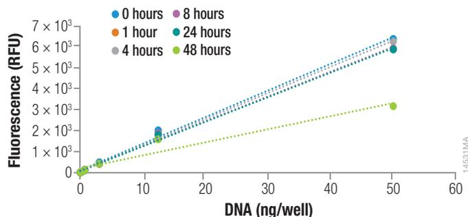
**Figure 2. QuantiFluor® dsDNA Dye working solution.** A 1:200 dilution working solution was left in a trough on the deck of a liquid handler exposed to ambient laboratory temperature and light. Dye was used at several time points to measure DNA in 384-well plate format over the range 0.05–50ng/well. A decrease in RFU signal was observed only after 24–48 hours.
