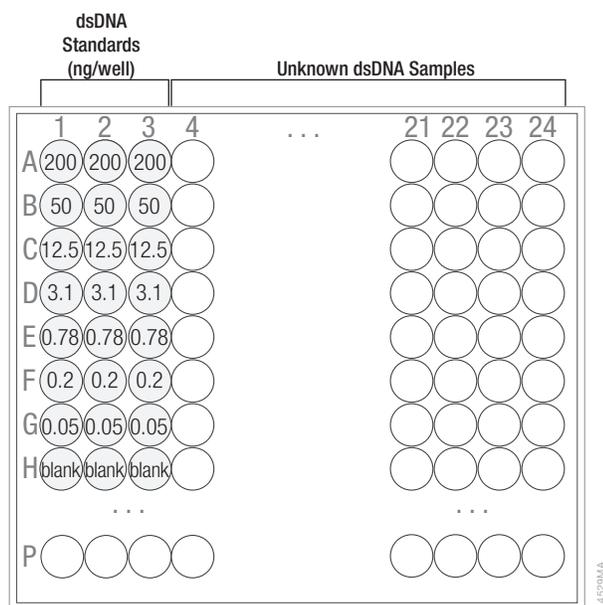
**Figure 1. Example 384-well plate map with standards, blanks and unknowns labeled.**
