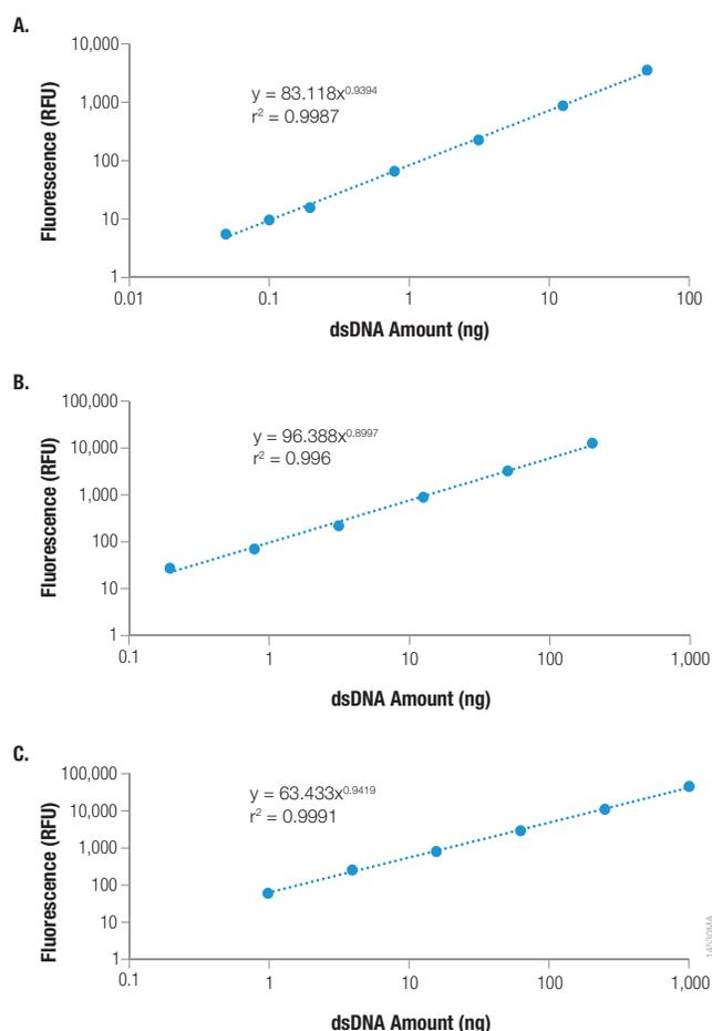
**Figure 3. QuantiFluor® dsDNA Dye at three different concentrations accurately quantitates DNA over a range of 0.05–1,000ng in 384-well format. Panel A. 0.2µl dye/well; Panel B. 1µl dye/well; Panel C. 3µl dye/well.**
