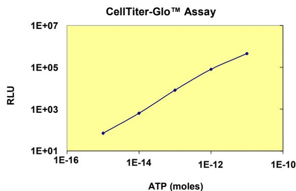
**Figure 1.** CellTiter-Glo<sup>®</sup> Assay on the GloMax<sup>®</sup> Multi Microplate Luminometer using ATP standards diluted in HEPES buffer.
