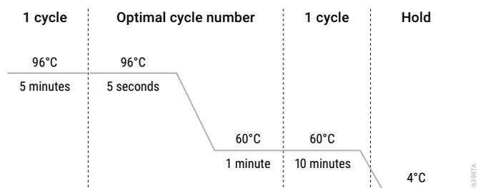
**Figure 2. Thermal cycling protocol for the ProFlex® PCR System.**
