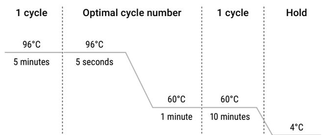
**Figure 1. Thermal cycling protocol for the ProFlex® PCR System.**
