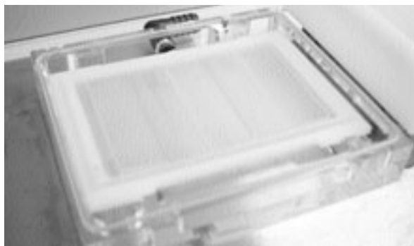
Figure 2. Picture of position A3 setup on the Beckman Coulter Biomek® 2000 Workstation. To optimize the Elution Plate height and ensure the filter plate nozzles are just within the wells of the Elution Plate, two Beckman Coulter spacers are required: a Spacer Filter Plate and Spacer Plate. The clear plastic Spacer Plate is placed on the white Spacer Filter Plate. The two are placed in the Vacuum Filtration Manifold Base.
