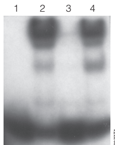
Figure 1. Gel shift assays. Gel shift assays were performed as described in Section 5. Lane 1, negative control ( ^{32}\text{P} -labeled SP1 Oligo without HeLa Nuclear Extract); lane 2, positive control (HeLa Nuclear Extract and ^{32}\text{P} -labeled SP1 Oligo); lane 3, HeLa Nuclear Extract with ^{32}\text{P} -labeled SP1 Oligo plus unlabeled SP1 Oligo (specific competitor); lane 4, HeLa Nuclear Extract with ^{32}\text{P} -labeled SP1 Oligo plus unlabeled AP2 Oligo (nonspecific competitor). DNA binding and electrophoresis conditions were as described in Section 5.
