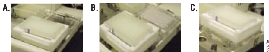
Figure 3. Example of vacuum manifold disassembly, placement of the Collection Plate and reassembly of vacuum manifold for elution of purified polyhistidine-tagged protein on the Beckman Biomek® 2000. Panel A. Disassembly of vacuum manifold. Panel B. Placement of Collection Plate. Panel C. Reassembly of vacuum manifold.
