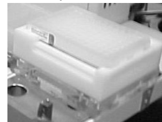
Figure 4. Vacuum manifold disassembly, placement of Elution Plate and reassembly of vacuum manifold for elution of purified amplification products on the Beckman Biomek® 2000.
