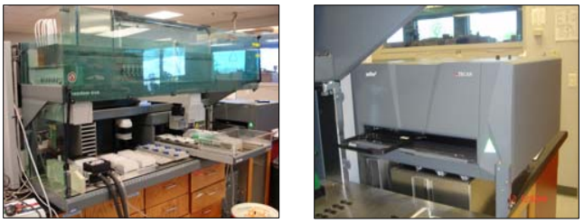
Tecan Freedom Evo® with 2 meter deck, 8-tip LiHa, and RoMa arm
