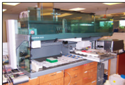
Fig. 1. The Tecan Freedom EVO® 200 system with 8-tip LiHa and RoMa arm, integrated with a TeMo™ and GENios Pro™ plate reader.
