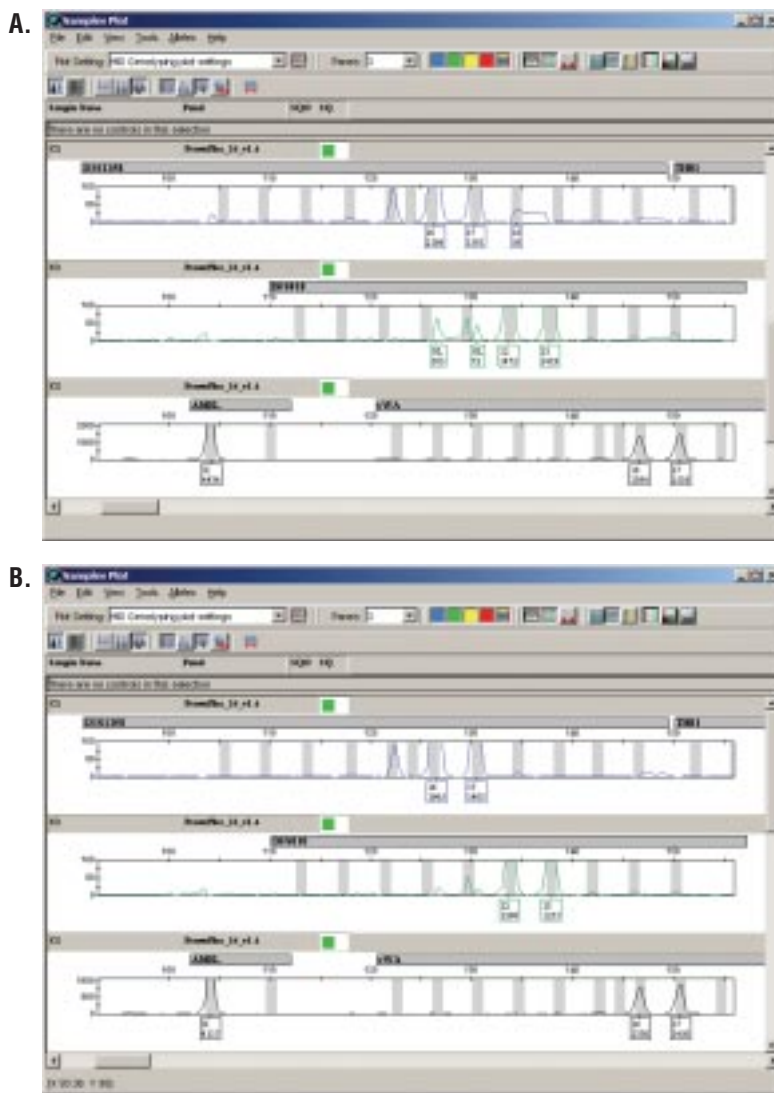
Figure 3. Close-up view of the sample “C1” from Figure 2 analyzed with a cutoff of 50RFU. Panel A. Current PowerPlex® Matrix Standards, 3100 (Cat.# DG3650). Panel B. The new PowerPlex® Matrix Standards, 3100—Custom (Cat.# X3121). Note the reduction of bleedthrough from the fluorescein channel into the JOE channel and the reduction of the raised baseline in the fluorescein channel caused by the JOE channel.
