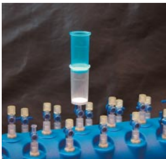
Figure 3. Proper assembly of the PureYield™ Clearing Column (blue) and the PureYield™ Binding Column (white) for use with the PureYield™ Plasmid Midiprep System vacuum protocol.
