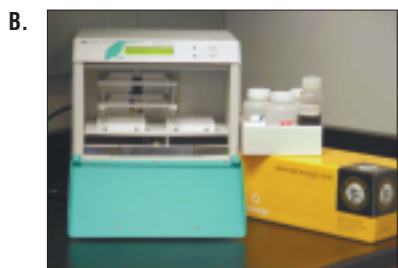
Figure 1. Isolation of DNA using the KingFisher™ instrument. Panel A: MagneSil™ Paramagnetic Particle (PMPs)-capture of genomic DNA. Panel B: KingFisher™ instrument.
