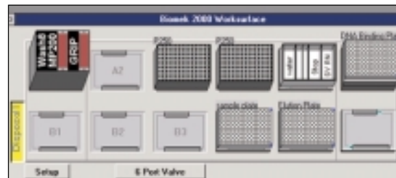
▲ Figure 2. Deck layout for performing RNA isolation on the Biomek® 2000 using the SV 96 Binding Plate.
