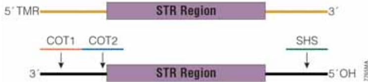
Figure 2: Schematic diagram of COT1, COT2 and SHS oligonucleotide hybridization to the vWA amplicon. The yellow line represents the TMR-labeled strand of the vWA amplicon. The black line represents the complementary unlabeled strand. The grey box denotes the location of short tandem repeats. The sites where the COT1, COT2 and SHS oligonucleotides anneal to the unlabeled strand are indicated.
