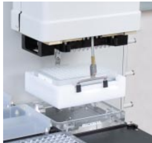
Automated isolation of total RNA using the SV 96 Total RNA Isolation System on the Beckman Coulter Biomek® FX.
