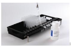
**Figure 2. Setup and configuration of the deck tray.** Elution Buffer is added to the elution tubes as shown. Plungers are in well #8 of the cartridge.
