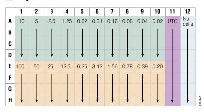
Figure 4. ApoLive-Glo™ Multiplex Assay plate layout following Steps 2-4.
