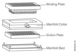
**Figure 2. Diagram of the Vac-Man® 96 Vacuum Manifold with the Wizard® SV 96 Plasmid DNA Purification System components.** Panels A, B and C show the manifold and plate combinations necessary to accomplish DNA binding, washing and elution, respectively.
