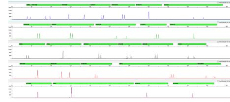
1-1.2mm punch of whole blood on FTA® paper amplified according to direct-amplification protocol (26-cycles). Separated on a 3500 Genetic Analyzer using a 1.2kV,15 second injection and a 13kV run voltage.
