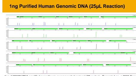
1ng of 2800M DNA amplified according to recommended protocol (29-cycles). Separated on a 3500 Genetic Analyzer using a 1.2kV, 15 second injection and a 13kV run voltage.
