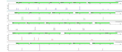
1-1.2mm punch of whole blood on FTA® paper amplified according to direct-amplification protocol (25-cycles) using AmpSolution™. Separated on a 3500 Genetic Analyzer using a 1.2kV,15 second injection and a 13kV run voltage.
