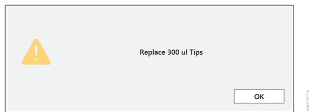
Figure 23. Insufficient tips on the system to complete a method. In the event that all tips of a given tip type are consumed during a run, the instrument will pause and unlock the door. Open the door, load more tips of the indicated type on the tip and plate carrier, close the door and press OK to resume processing.
